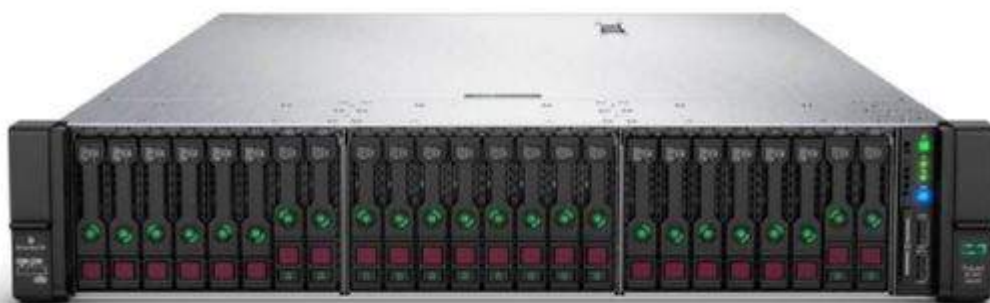
24 SFF (incl 12 NVMe SSDs) hot-plug drive model
